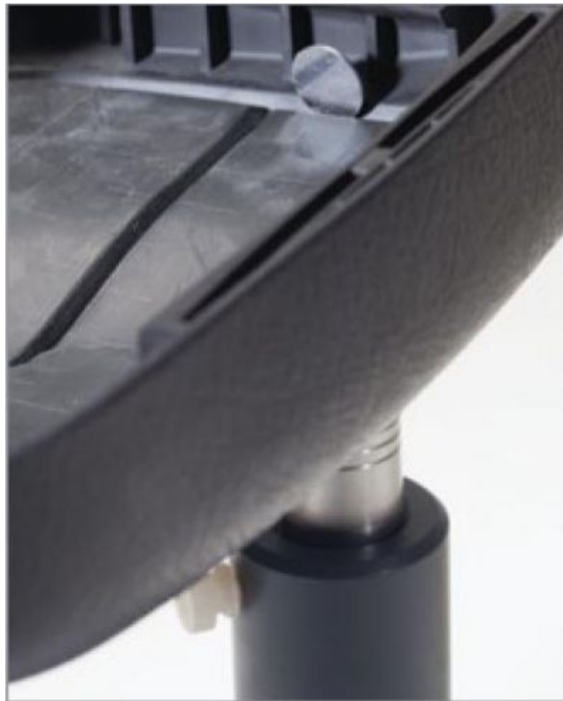
Figure 2. Probe placement on the outside of an air bag cover.
