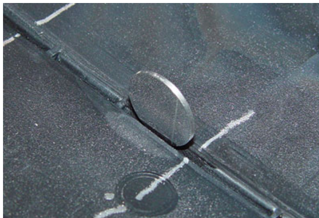
Figure 3. Target disk placement inside a tear seam.
